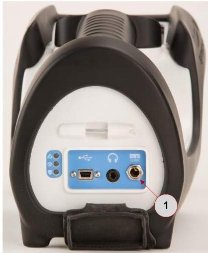
Figure 21: Location of the Power Receptacle
