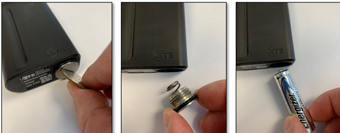
Figure 4: Unscrewing (left) and Removing the Battery Cover (center), and Replacing the Battery (right)
