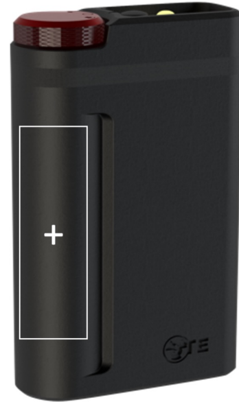
Figure 1: Radiation Pager Detector Location and Center
