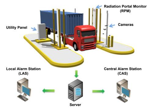
The NSDD-provided radiation detection system typically consists of the elements pictured above including:
