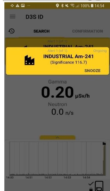
If more than one isotope is detected, an indication “Alert 1 (of 2)” will be displayed on the pop-up window. Swipe to the left to display the next alert.
