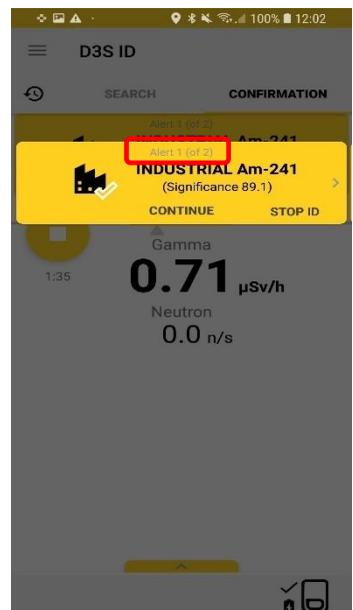
Visual notification panel of the alert will remain displayed. If more than one isotope is detected, an indication “Alert 1 (of 2)” will be displayed on the pop-up window. Swipe to the left to display the next alert.
